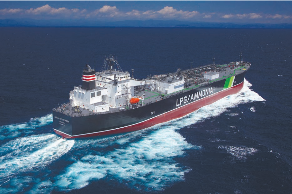
An illustration depicts the Luna Pathfinder, a large liquefied petroleum gas carrier equipped with a dual-fuel LPG-ammonia engine, which is scheduled to set sail in 2026. NYK
