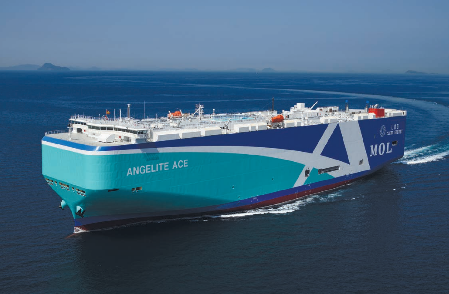
The Angelite Ace is a liquefied natural gas-fueled car carrier capable of carrying 7,000 car equivalent units.
