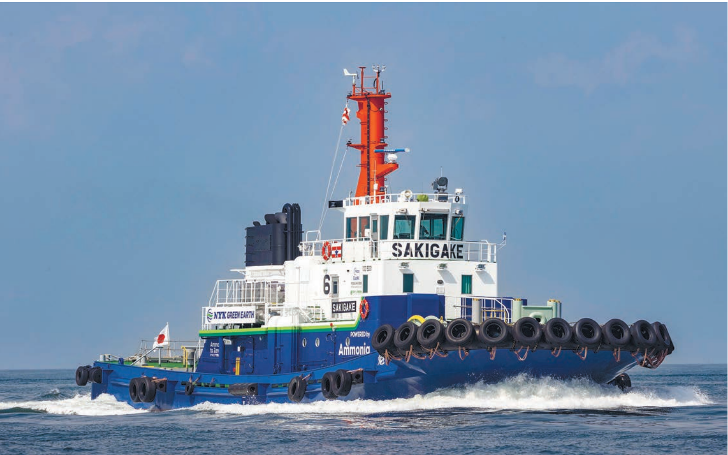
The Sakigake is the world's first ammonia-fueled tugboat. NYK
