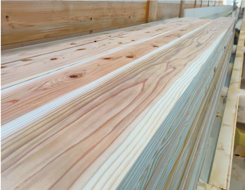
Sugi is straight-grained, soft and easy to process.
