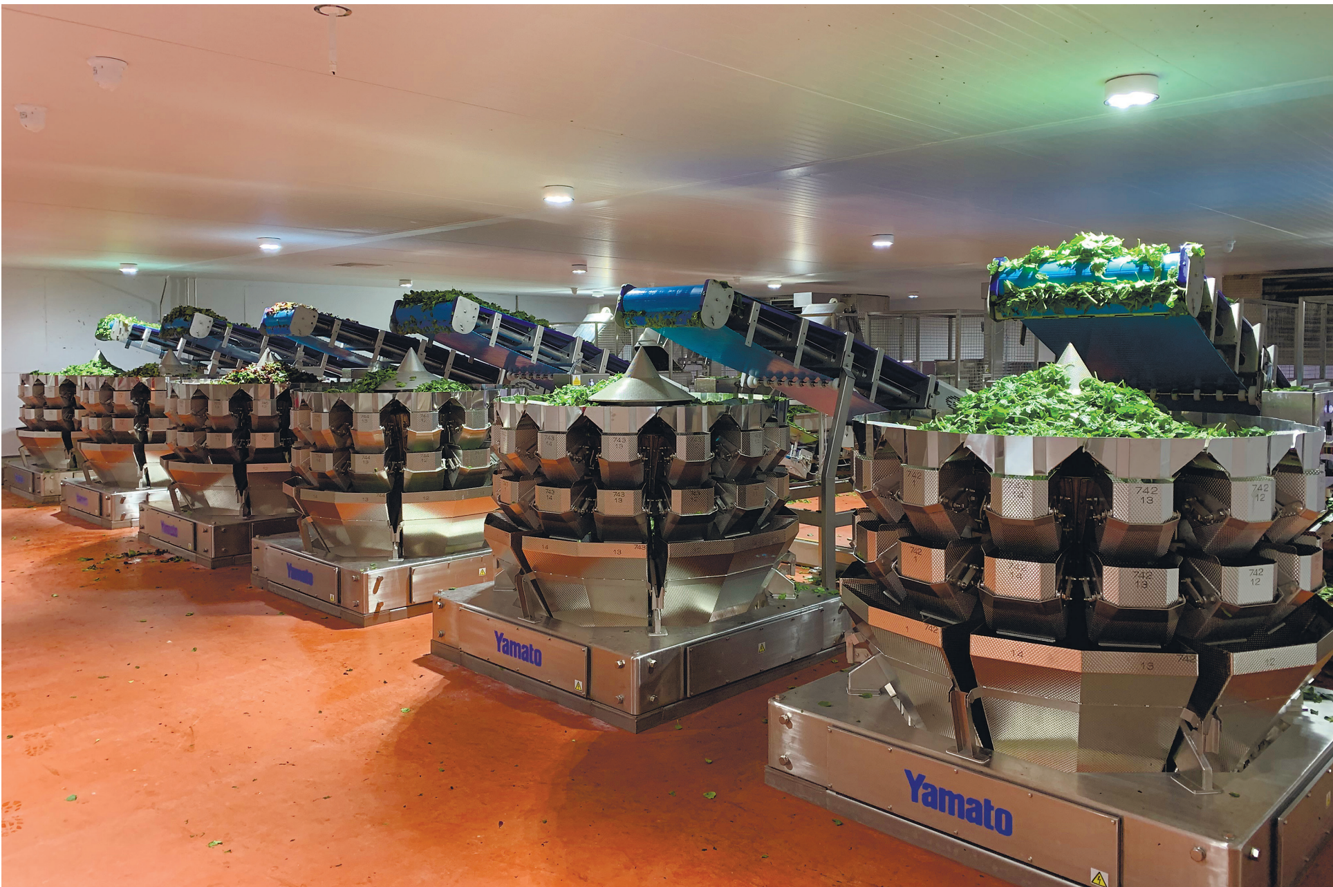
Dataweigh combination scales precisely distribute salad at a large produce factory. YAMATO SCALE CO. LTD.
