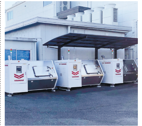
The YC100 composter is used in Japan to recycle food waste as part of resource-recycling initiatives.
