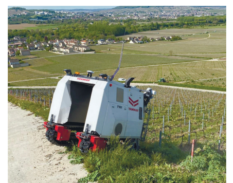
Left: Yanmar makes a variety of battery-powered construction equipment. Right: The YV01 spraying robot is designed for vineyards, which often have steep slopes that make cultivation dangerous.
