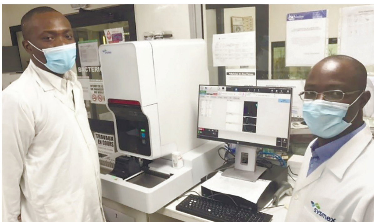
Technicians are able to test blood for malaria using the Sysmex XN-31 analyzer. SYSMEX
